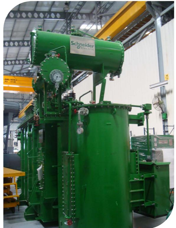
*Tata Power's new 20MVA design achieves continuous loading of 25/30MVA (KNAN/KNAF) for 25% capacity increase in a space constrained area.*
