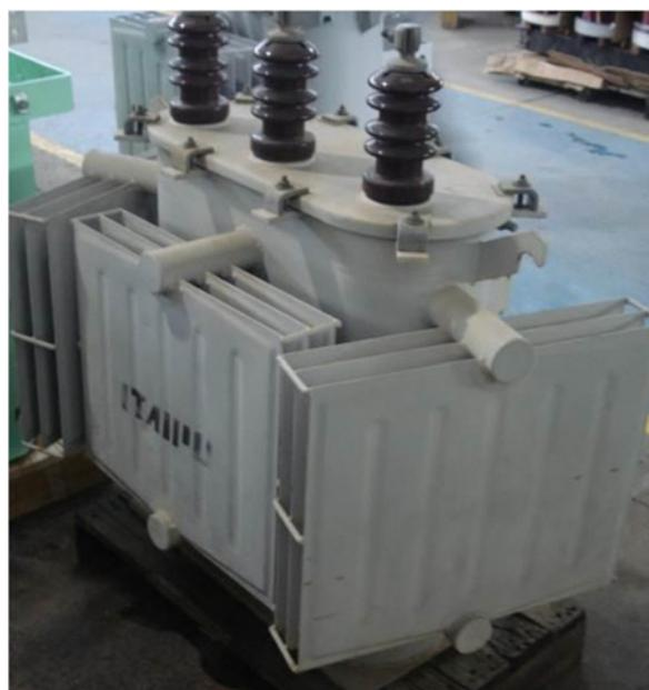
**Fig. 1** Overview of the prototype transformer after 12 years of continuous service at overhead distribution lines in Brazil
