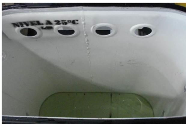
**Fig. 3** View of tank bottom, after removal of active parts and fluid
