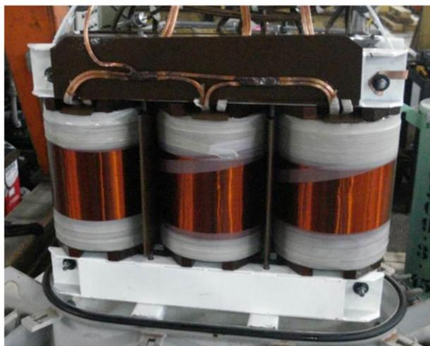
**Fig. 4** Core and coil assembly immediately after untanking
