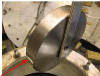
Detail showing the 216 mm diameter x 38 mm thick with a edge radius of 4.3 mm installed below a 550kV (BIL 1800kV) bushing
